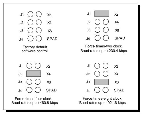
Figure 4 --- Clock multiplier jumper options
